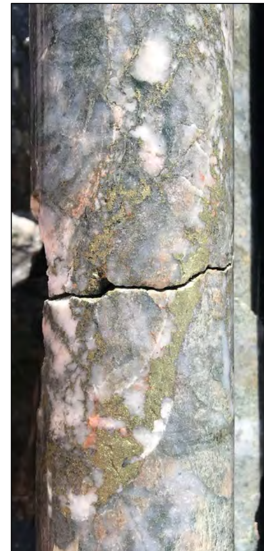
Anagulu Gold-Copper Porphyry Prospect - highly mineralised breccia with chalcopyrite in AND005
