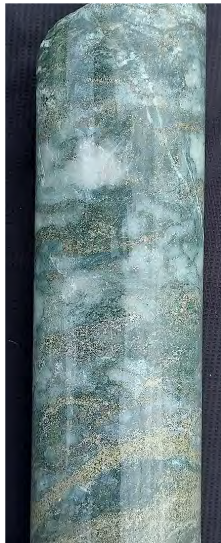
Aburna Orogenic Gold Prospect - highly mineralised quartz breccia with pyrite
