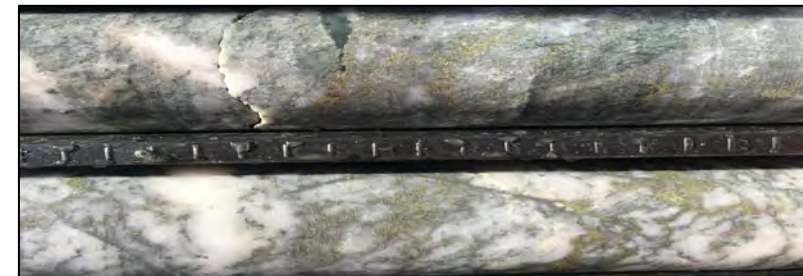
Chalcopyrite rich drill core from Anagalu
