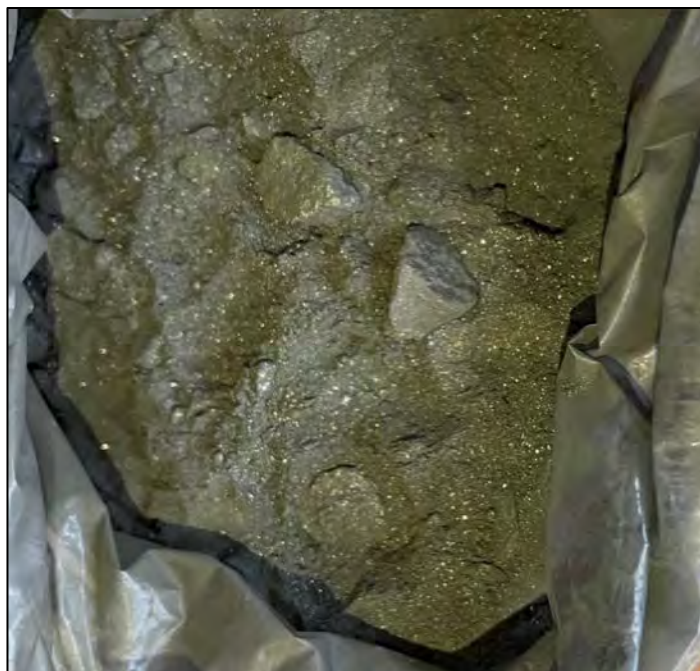
Massive sulphide from RC drilling at Tolegimja
