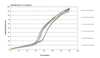
Six 1m bioleach amenability columns on 4.75mm, 3.35mm and 2.36mm material show 89% to 96% copper dissolution after 140 days.
